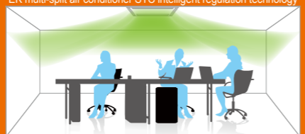
When return air temperature of indoor unit is close to set temperature of air conditioning, it's necessary to intelligently increase vaporization temperature of indoor unit, so as to avoid discomfort caused by direct blowing of cold air.
