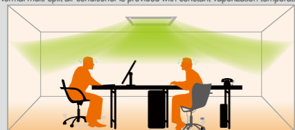
With constant indoor vaporization speed, although temperature is reduced at a low speed, it's still hot in the room.
