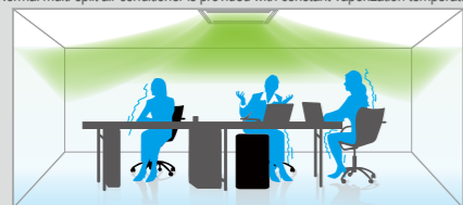
When return air temperature of indoor unit is close to set temperature of air conditioning, vaporization temperature of indoor unit is low, which often causes discomfort caused by direct blowing of cold air.
